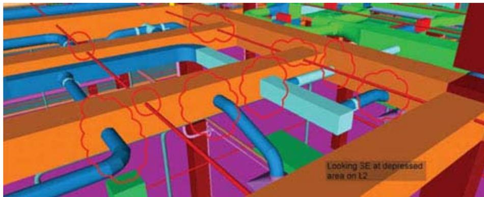
Bringing together design and contractor’s models allowed for real time clash detection — conflicts are resolved virtually prior to any work starting in the field.
