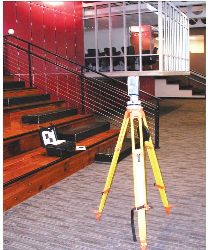
A tripod-mounted laser sends out a light beam to record the coordinates of the surrounding surfaces.
